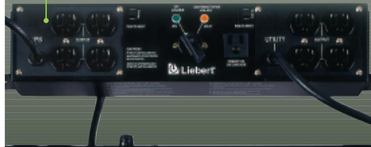
The Liebert 2U POD has two modes of operation, UPS mode (UPS available) and utility mode (maintenance bypass). During the UPS mode, the power is being routed through the UPS system as per Figure 1. During the utility mode of operation, power is being routed around (bypassing) the UPS system as per Figure 2, with power being supplied to the connected load through the Liebert 2U POD.
